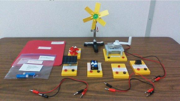
Demonstrates the conversion between different forms of energy. It includes four devices for generating electrical energy from mechanical motion (hand generator), chemical energy (batteries), light (solar cell) and wind (windmill) and three devices for using electrical energy to generate light (LED) motion (motor) and sound (buzzer).
